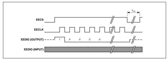
**EWEN (Erase/Write Enable):** Enables the EEPROM for erase and write operations. The EEPROM will allow erase and write operations until the "Erase/Write Disable" command is sent, or until power is cycled.
