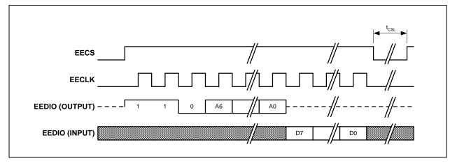
**WRITE (Write Location):** If erase/write operations are enabled in the EEPROM, this command will cause the contents of the E2P\_DATA register to be written to the EEPROM location selected by the EPC Address field (EPC\_ADDR). The EPC\_TO bit is set if the EEPROM does not respond within 30ms.
