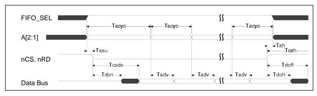
FIGURE 6-4: RX DATA FIFO DIRECT PIO BURST READ CYCLE TIMING
