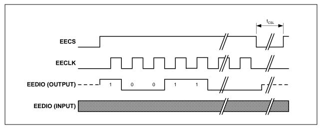
**READ (Read Location):** This command will cause a read of the EEPROM location pointed to by EPC Address (EPC\_ADDR). The result of the read is available in the E2P\_DATA register.
