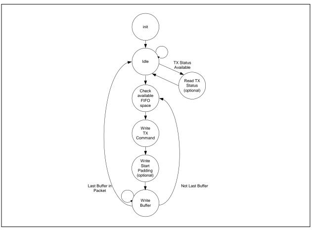
FIGURE 3-12: SIMPLIFIED HOST TX FLOW DIAGRAM
