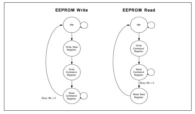
The host can disable the EEPROM interface through the GPIO\_CFG register. When the interface is disabled, the EEDIO and ECLK signals can be used as general-purpose outputs, or they may be used to monitor internal MII signals.
