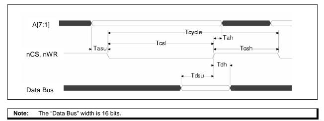
FIGURE 6-5: PIO WRITE CYCLE TIMING
