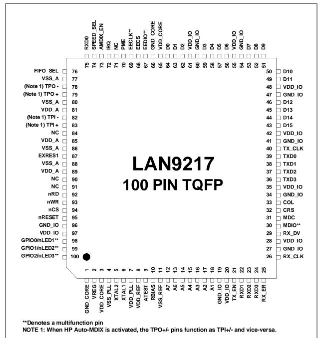
FIGURE 2-1: PIN CONFIGURATION (TOP VIEW)
