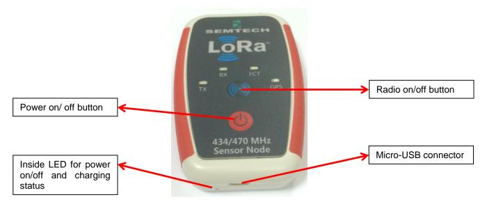
Figure 1: keyboard and connector of LoRa sensor node
