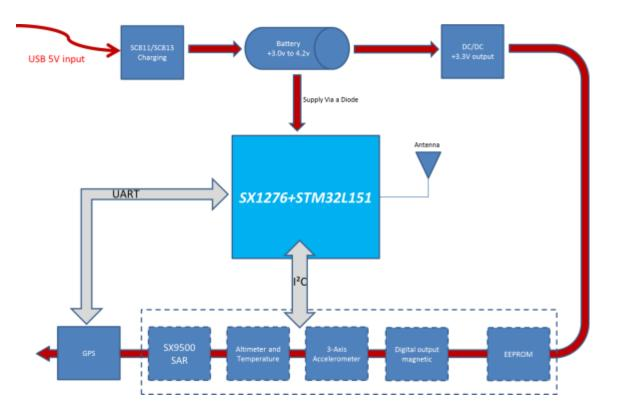
Figure 2: Block diagram of LoRa sensor node
