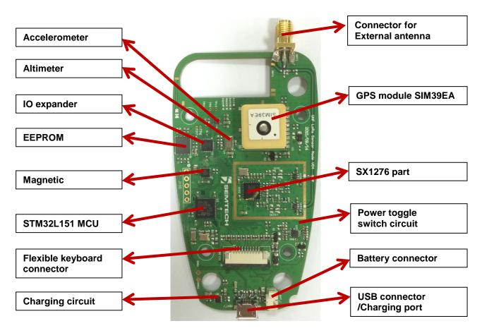
(Top side) Figure 3: HW arrangement of layout-Top layer
