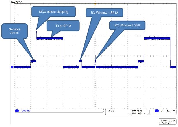
Figure 19: RF module Energy Profile
