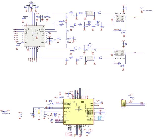
Figure 6 LoRa sensor node Schematics\_2—RF+MCU part
