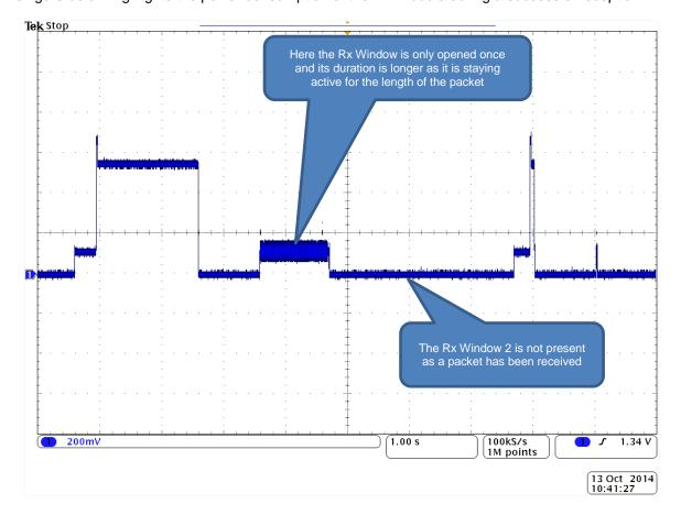
The figure below highlights the power consumption of the RF module during a successful reception.
