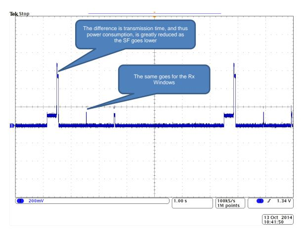
Figure 22: Power Consumption at SF7
