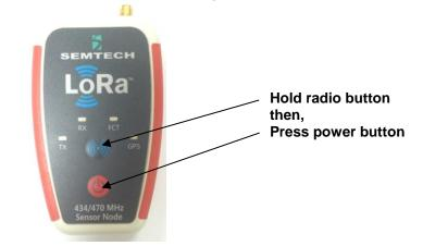
Figure 9: How to enter bootloader mode with LoRa Sensor Node
