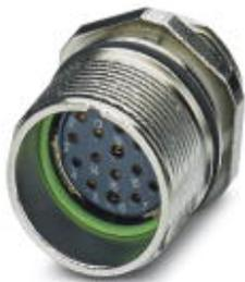
Device connector for front wall, straight, shielded: yes, SPEEDCON locking, M23, No. of pos.: 16+2+PE, type of contact: Socket, Crimp connection, Axial seal, Central fastening Pg13,5
