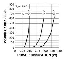
Figure 5. Copper Area vs. Power SOIC Power Dissipation (T<sub>A</sub>)
