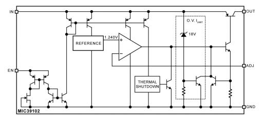
MIC39102 Adjustable Regulator Block Diagram
