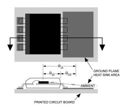
Figure 3. Thermal Resistance
