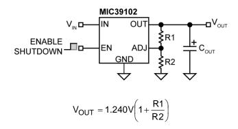
Figure 2. Adjustable Regulator with Resistors
