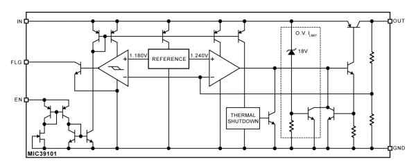
MIC39101 Fixed Regulator with Flag and Enable Block Diagram
