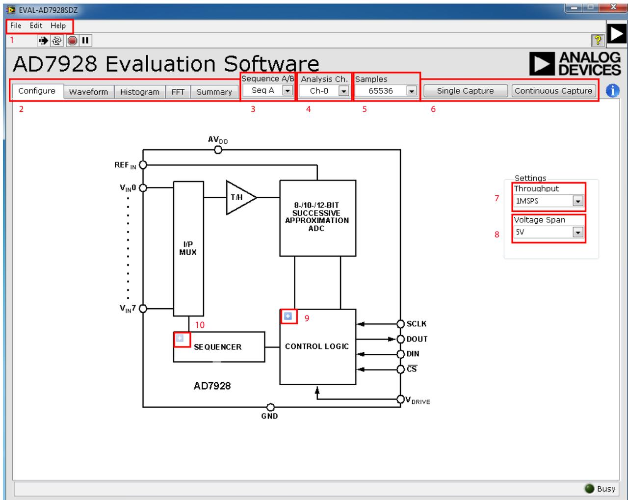
Figure 13. AD7928 Evaluation Software Main Window
