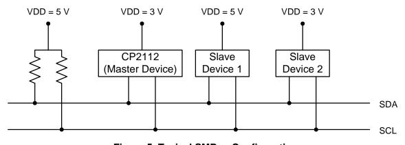
Figure 5. Typical SMBus Configuration
