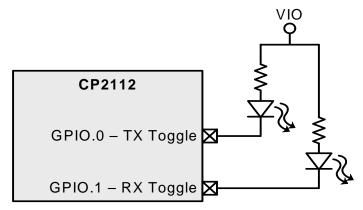
Figure 9. Transmit and Receive Toggle Typical Connection Diagram
