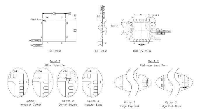
Figure 3. QFN-24 Package Drawing
