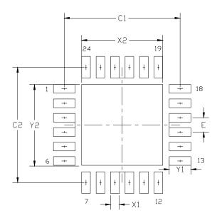
Figure 4. QFN-24 Recommended PCB Land Pattern
