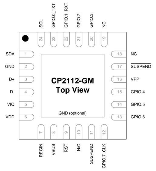
Figure 2. QFN-24 Pinout Diagram (Top View)
