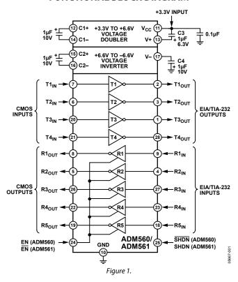
device begins communication. The active receivers alert the processor, and then take the ADM560 out of shutdown mode.
