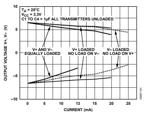
Figure 10. V+, V- vs. Load Current
