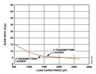
Figure 8. Transmitter Slew Rate vs. Load Capacitance
