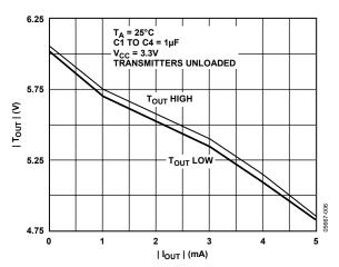
Figure 5. Transmitter Output Voltage vs. Load Current
