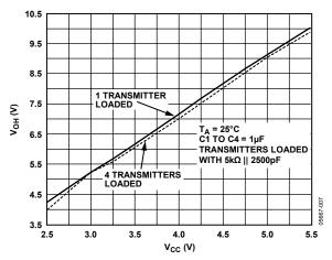
Figure 6. Transmitter Output Voltage High vs. Vcc
