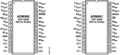
Figure 2.ADM560 Pin Configuration
