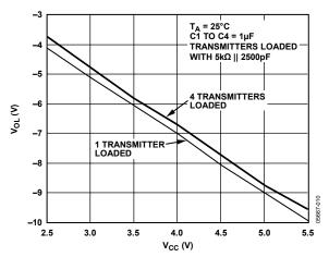
Figure 9. Transmitter Output Voltage Low vs. Vcc
