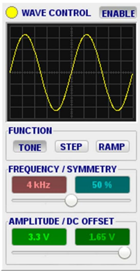
The waveform generator in BS05 itself is completely arbitrary; it can replay any wavetable of up to 1024 sample points programmed into it.
