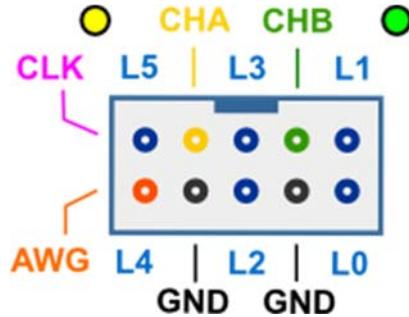
It's conveniently arranged so the two ground pins can pair with the analog inputs, waveform and clock generator outputs or logic inputs L0, L2 and L4.
