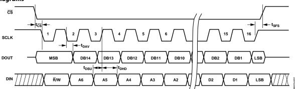
Figure 2. SPI Timing and Sequence
