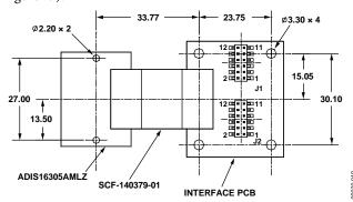
Figure 19. Physical Diagram for Mounting the ADIS16305/PCBZ
