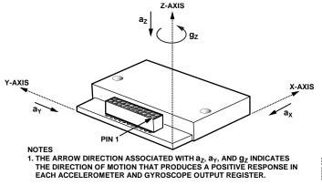
Figure 6. Axial Orientation
