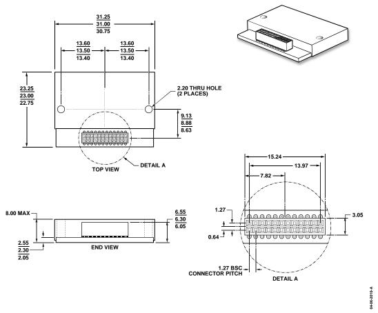
Figure 21. 24-Lead Module with Connector Interface (ML-24-4) Dimensions shown in millimeters
