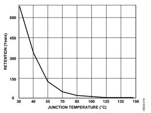
Figure 18. Flash/EE Memory Data Retention
