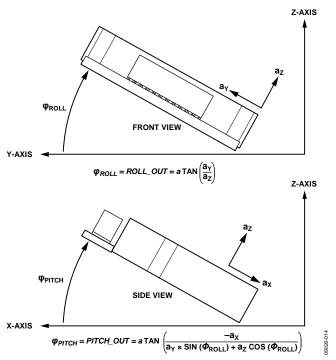
Figure 14. Orientation for PITCH\_OUT and ROLL\_OUT Angles
