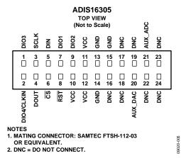
Figure 5. ADIS16305 Pin Configuration
