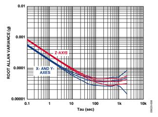
Figure 8. Accelerometer Allan Variance
