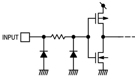
Figure 8. Input Equivalent Circuit
