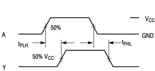
Figure 4. Switching Waveforms
