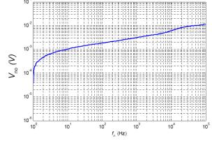
Figure 2: Output noise voltage spectral density
