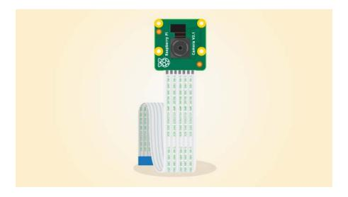
The Raspberry Pi camera module v2 replaced the original camera module in April 2016. The v2 camera has a Sony IMX219 8-megapixel sensor (compared to the 5-megapixel OmniVision OV5647 sensor of the original camera).
