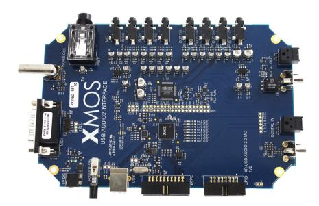
Figure 1: USB Audio 2.0 MC reference design board
