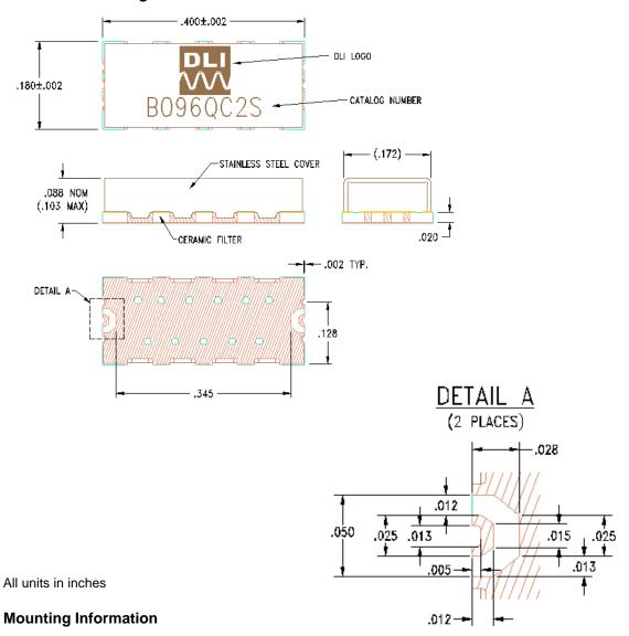
PCB ground pattern length and width can be 0.002-0.003 inches larger than filter footprint. Dimensions of filter launch and PCB launch pattern should be closely matched.
