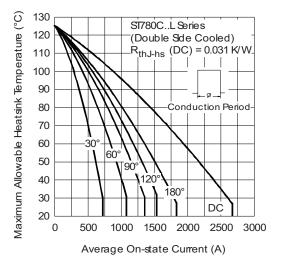
Fig. 4 - Current Ratings Characteristics
