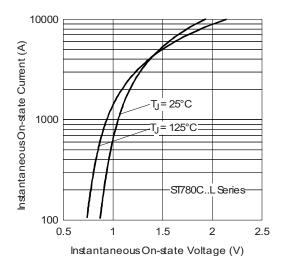
Fig. 9 - On-State Voltage Drop Characteristics
