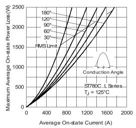
Fig. 5 - On-State Power Loss Characteristics
