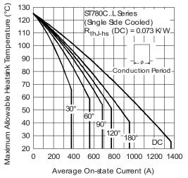
Fig. 2 - Current Ratings Characteristics
