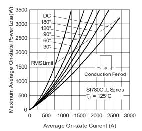
Fig. 6 - On-State Power Loss Characteristics
