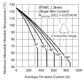
Fig. 1 - Current Ratings Characteristics
