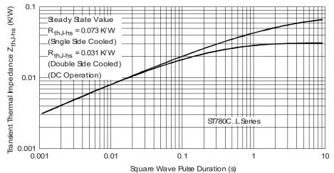
Fig. 10 - Thermal Impedance  $Z_{thJ\text{-}hs}$  Characteristics
