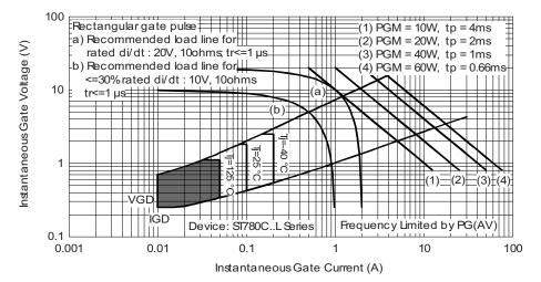
Fig. 11 - Gate Characteristics
