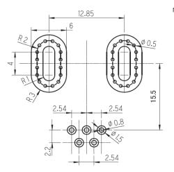
Note) If 2 or more trace layers are used as the current path, please make enough number of through-holes to flow current between the trace layers.
