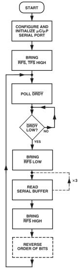
Figure 15. Flowchart for Continuous Read Operations to the AD7711A
