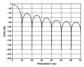
Figure 6. Frequency Response of AD7711A Filter
