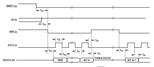
Figure 12b. External Clocking Mode, Output Data Read Operation (RFS Returns High during Read Operation)
