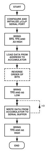
Figure 16. Flowchart for Single Write Operation to the AD7711A
