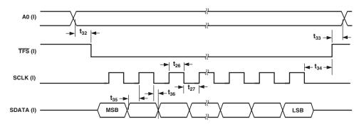
Figure 13a. External Clocking Mode, Control/Calibration Register Write Operation
