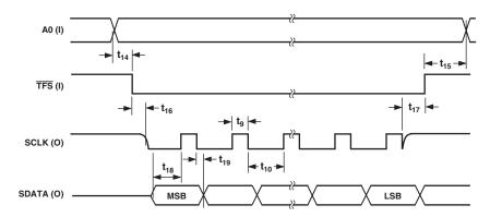
Figure 11. Self-Clocking Mode, Control/Calibration Register Write Operation
