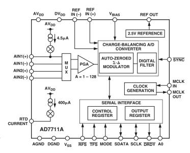
CMOS construction ensures low power dissipation, and a soft-ware programmable power-down mode reduces the standby power consumption to only 7 mW typical. The part is available in a 24-lead, 0.3 inch-wide, hermetic dual-in-line package (CERDIP), as well as a 24-lead small outline (SOIC) package.
