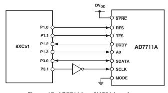
Figure 17. AD7711A to 8XC51 Interface
