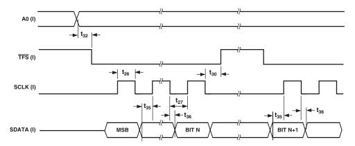
Figure 13b. External Clocking Mode, Control/Calibration Register Write Operation (TFS Returns High during Write Operation)
