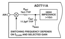
Figure 7. Analog Input Impedance
