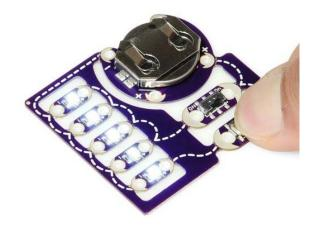
At this point you've probably become aware of the different functionality of each of the switches on the E-Sewing Kit. The button is a "momentary switch", meaning it's closed circuit-ness is fleeting, it only conducts when the button is actuated. The state of the Slide Switch is relatively permanent, until slid in the other direction the switch will remain either on or off.
