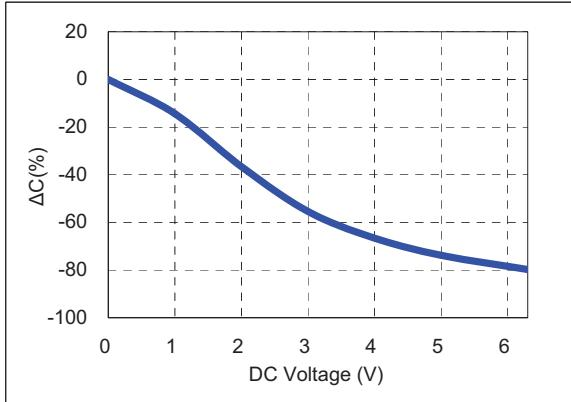
4) Bias TCC characteristics (Agilent 4284A, 1kHz, 0.5Vrms, 3.15Vdc)
