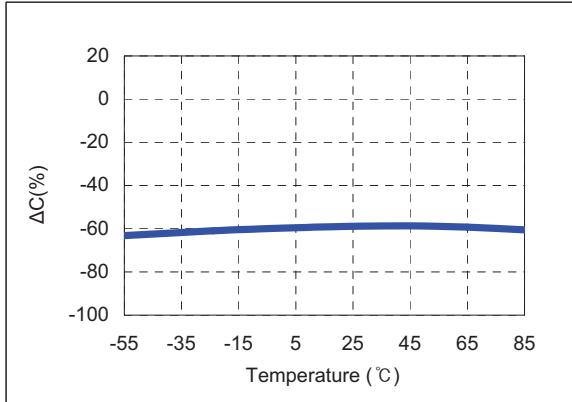
5) AC voltage characteristics (Agilent 4284A, 1kHz)
