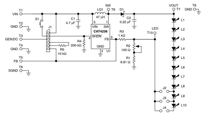
Figure 1. CAT4238AEVB Board Schematic
