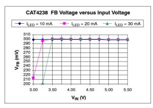
Figure 5. V<sub>FB</sub> Voltage Line Regulation
