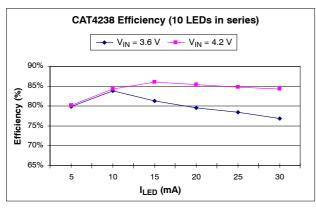
Figure 6. CAT4238 Efficiency Driving 10 LEDs in Series
