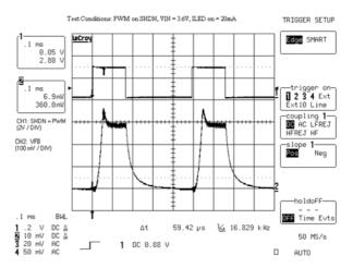
Figure 7. FB Voltage Waveform with PWM
