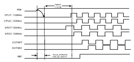
Figure 4. Power Down Deassertion Timing Waveform
