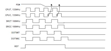
Figure 3. Power Down Assertion Timing Waveform
