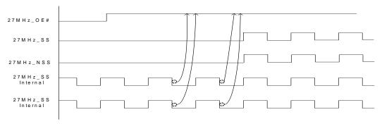
Figure 7. 27M\_OE# Deassertion Waveform
