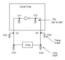
Figure 2. Crystal Loading Example
