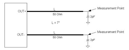
Figure 10. 0.7V Differential Load Configuration
