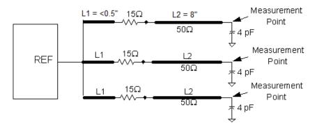
Figure 8. Single-ended REF Triple Load Configuration
