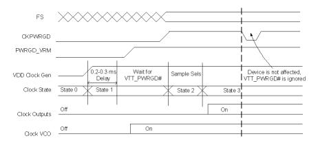
Figure 5. CKPWRGD Timing Diagram
