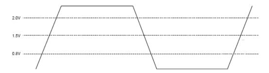
Figure 9. Single-ended Output Signals (for AC Parameters Measurement)
