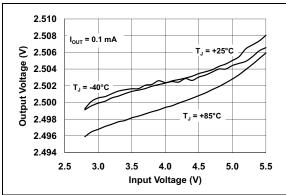
FIGURE 2-2: Output Voltage vs. Input Voltage ( $V_R$  = 2.5V).
