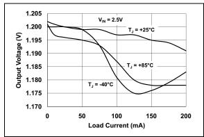
**FIGURE 2-4:** Output Voltage vs. Load Current ( $V_R = 1.2V$ ).
