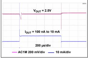
**FIGURE 2-14:** Dynamic Load Step  $(V_R = 2.5V)$ .
