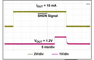
**FIGURE 2-22:** Start-up from SHDN  $(V_R = 1.2V)$ .
