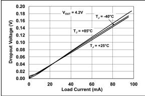
**FIGURE 2-8:** Dropout Voltage vs. Load Current ( $V_R = 4.2V$ ).
