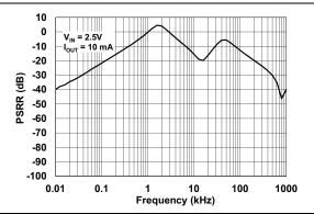
**FIGURE 2-10:** Power Supply Ripple Rejection vs. Frequency ( $V_R = 1.2V$ ).
