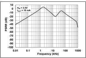
**FIGURE 2-11:** Power Supply Ripple Rejection vs. Frequency ( $V_R = 2.5V$ ).
