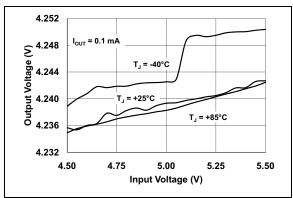
**FIGURE 2-3:** Output Voltage vs. Input Voltage ( $V_R = 4.2V$ ).
