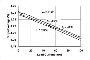
**FIGURE 2-6:** Output Voltage vs. Load Current ( $V_R = 4.2V$ ).
