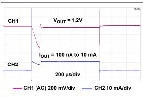
**FIGURE 2-13:** Dynamic Load Step  $(V_R = 1.2V)$ .
