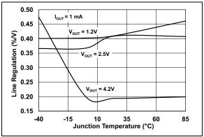
FIGURE 2-28:Line Regulation vs. JunctionTemperature.
