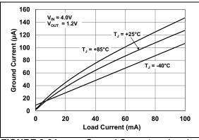
FIGURE 2-31: Ground Current vs. Load Current.
