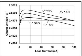
**FIGURE 2-5:** Output Voltage vs. Load Current ( $V_R = 2.5V$ ).
