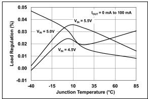
**FIGURE 2-27:** Load Regulation vs. Junction Temperature ( $V_R = 4.2V$ ).
