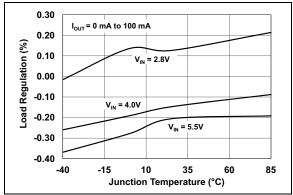
**FIGURE 2-26:** Load Regulation vs. Junction Temperature ( $V_R = 2.5V$ ).
