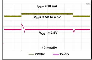
**FIGURE 2-17:** Dynamic Line Step  $(V_R = 2.5V)$ .
