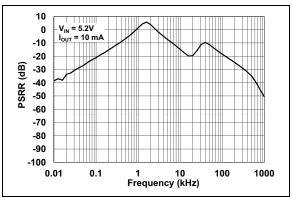
**FIGURE 2-12:** Power Supply Ripple Rejection vs. Frequency ( $V_R = 4.2V$ ).
