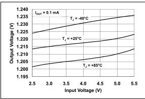
**FIGURE 2-1:** Output Voltage vs. Input Voltage ( $V_R = 1.2V$ ).
