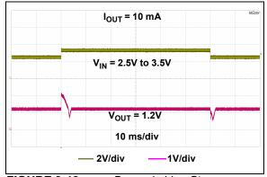
**FIGURE 2-16:** Dynamic Line Step  $(V_R = 1.2V)$ .
