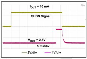
**FIGURE 2-23:** Start-up from  $\overline{SHDN}$  ( $V_R = 2.5V$ ).
