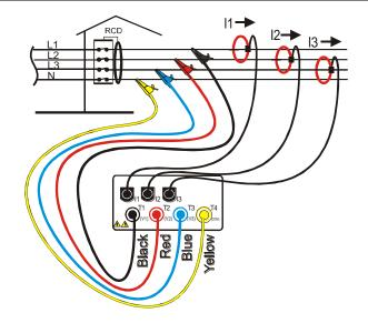
Instrument connection in a three phase 4-wire system
