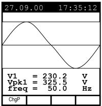
Example of screen in Example of screen in "3single-phase system wire" three-phase system
