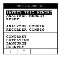
It's not possible to enter the **MENU** during a recording or a Real Time Energy measurement. Pressing this button during a recording will display the main recording parameters (see paragraph 10.2).
