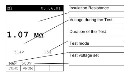
In order to evaluate the test you must compare the result with the limits indicated in the Guidelines (see Table1).
