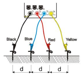
Instrument connection for Earth resistivity measurement
