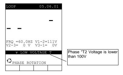
In the "Q" mode, if the instrument detects two phases connected together it displays the screen to the right.
