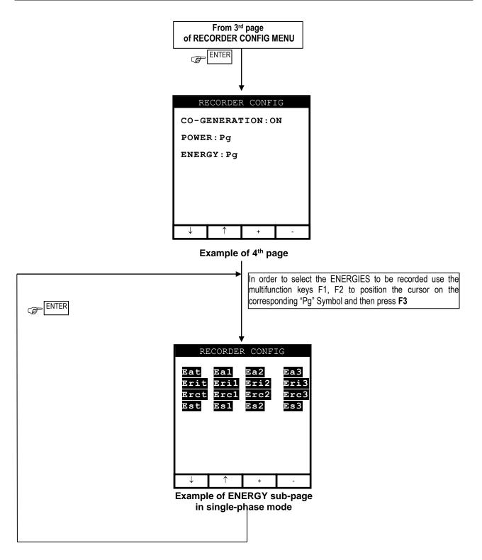
Selecting/deselecting the active energies for the recording, the corresponding active powers will be automatically selected/deselected.
