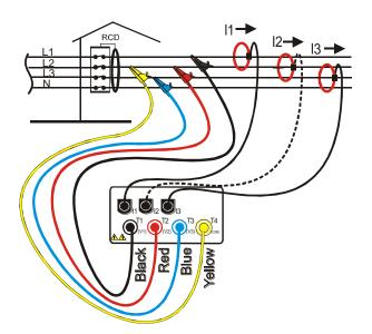
Instrument connection in a three-phase 3-wire system
