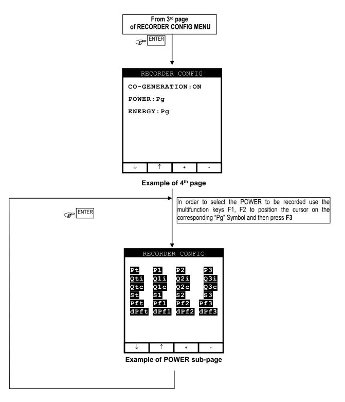
Selecting the active powers for the recording, the corresponding active energies will be automatically selected.
