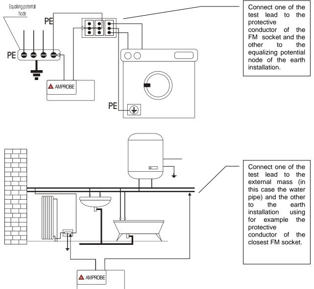
Examples for continuity measurement on conductors
