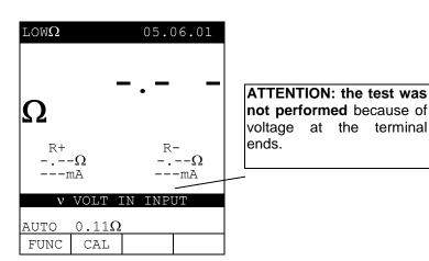
In the case that: RCALIBRATION>RMEASURED the instrument displays the screen to the right.
