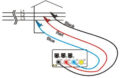
Instrument connection for Phase Sequence Detection in a 400V three-phase system
