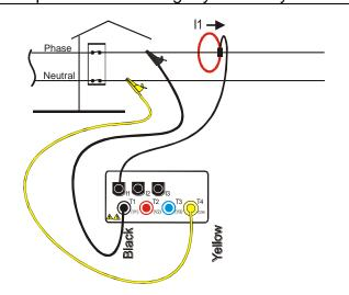
Instrument connection in a single-phase system
