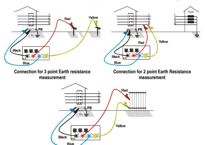
Connection for measuring the resistance between an extraneous conductive part and the earth system
