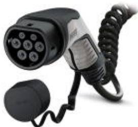
AC charging cable with Vehicle Connector, open cable end, with protective cap, Type 2, IEC 62196-2, 32 A / 250 V (AC), design line C-Line, cable: 4 m, black, spiraled, mating face: black, handle area: gray
