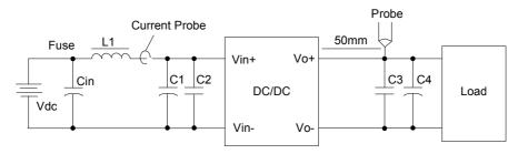
Figure 16 Ripple & noise test configuration
