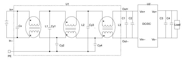
Figure 17 EMC test configuration
