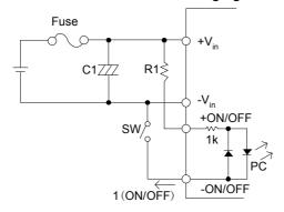
Figure 12 Connection of remote ON/OFF control (A)
