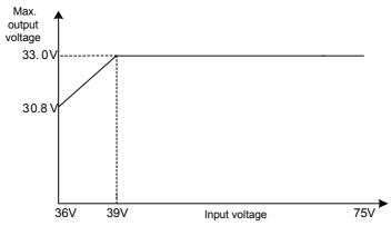
Figure 15 Trim-up-able voltage vs. input voltage
