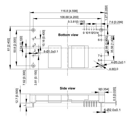
Unit: mm[inch] Bottom view: pin on upside Tolerance: X.Xmm±0.5mm[X.X in.±0.02in.] X.XXmm±0.25mm[X.XX in.±0.01in.]
