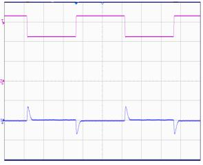
Figure 5 Dynamic response for 25% load step (50%  $\sim$  75%  $\sim$  50%) and 0.1A/ $\mu$ s slew rate, see Figure 11 for test configuration. CH1-output voltage (500mV/div); CH2-output current (5A/div)
