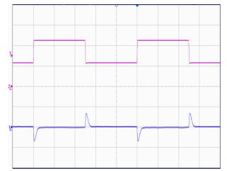
Figure 4 Dynamic response for 25% load step (25%  $\sim$  50%  $\sim$  75%) and 0.1A/ $\mu$ s slew rate, see Figure 11 for test configuration, CH1-output voltage (500mV/div); CH2-output current (5A/div)
