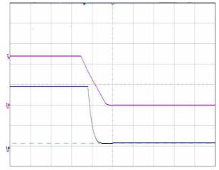
Figure 7 Output voltage shut down by power off, (5ms/div), see Figure 11 for test configuration, CH2-input voltage (20V/div); CH1-output voltage (10V/div)
