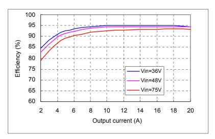
Figure 1 Efficiency vs. output current, T<sub>a</sub>=25°C, T<sub>c</sub>=40°C, V<sub>o</sub>=30V
