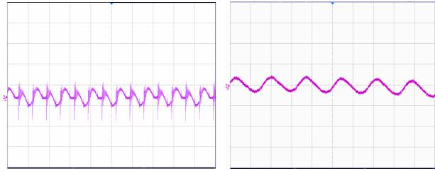
Figure 2 Output ripple & noise (5 $\mu$ s/div, 50mV/div), see Figure 16 for test configuration
