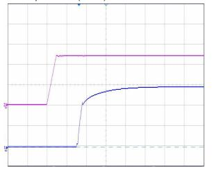
Figure 6 Output voltage startup by power on, (5ms/div), see Figure 11 for test configuration, CH2-input voltage (20V/div); CH1-output voltage (10V/div)
