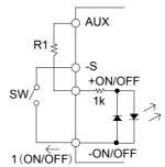
Figure 13 Connection of remote ON/OFF control (B)
