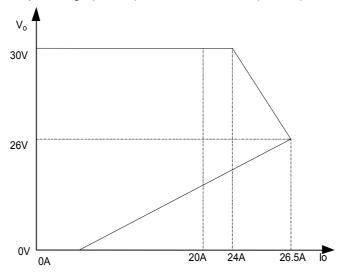
Figure 10 Over-current protection characteristics
