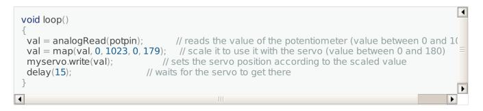
Without feedback, most servo programming has to make some assumptions about how long a particular move will take. Adding fixed-time delays to servo code works OK for simple applications, but can result in slow and/or jerky performance when trying to coordinate multiple servo motions or interactions between servos and other sensors or actuators.
