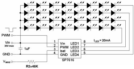
Figure 1. Evaluation Board Schematic Diagram for SP7616
