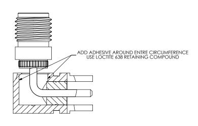
IN-PROCESS 4 ADD ADHESIVE TO BODY F:\DWG\MISC\MKTG\SMA-J-P-X-RA-TH1-MKT.SLDDRW
