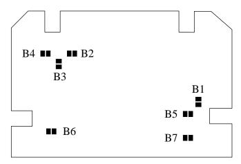
Fig.3 - Solder Bridge Link Selection Of Input Range
