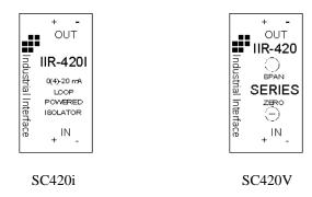
Fig. 2 - Front Panel Labels
