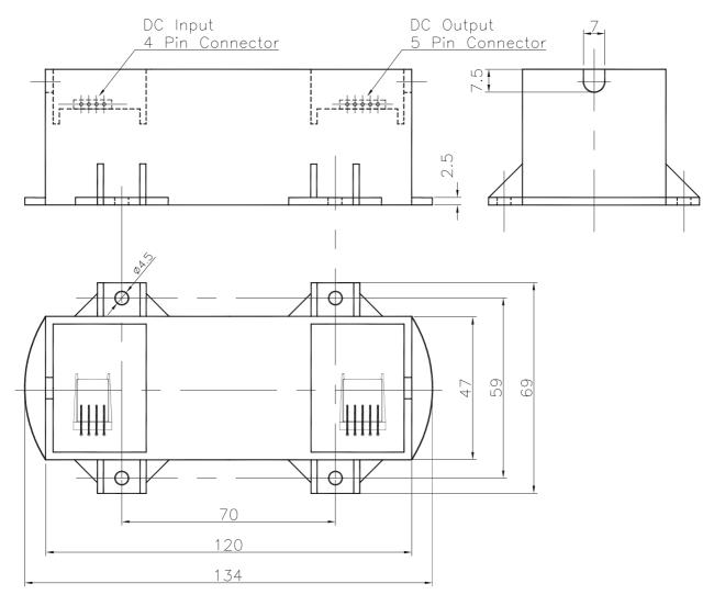
Fig. 2 Mechanical Drawing ISO3116I
