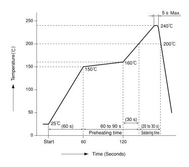
Applicable Conditions Reflow system: IR reflow Solder type: Cream type 63 Sn/37 Pb (Flux component 9 wt%) Test board: Glass epoxy 85 x 60 x 1 mm Metal mask thickness: 0.15 mm
