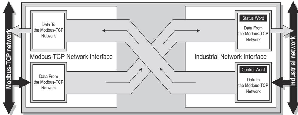
Each buffer holds a maximum of 256 bytes of data. The first two I/O mapped bytes in either direction can be dedicated for control/status information, and another eight bytes of data coming from the Modbus-TCP network can feature a live list. Please note that the actual number of bytes that can be exchanged is highly network dependent.
