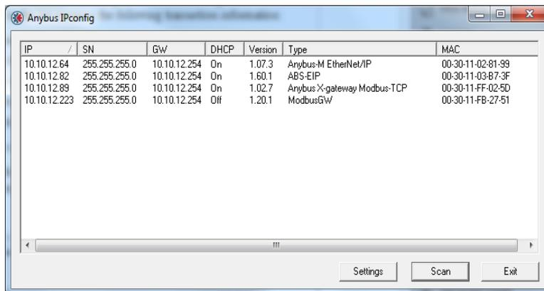
If a list of connected devices does not show automatically, press the scan button. Identify the IP address of the X-gateway by its type 'Anybus X-gateway Modbus-TCP' or by its MAC address. The MAC address of the X-gateway can be found at the bottom of the module.
