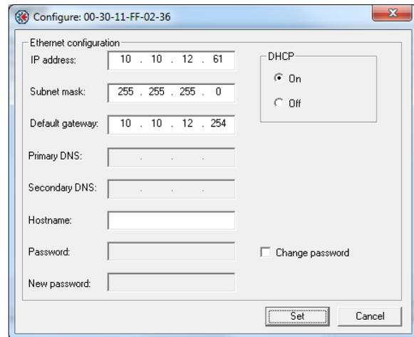
In the configuration window the TCP/IP settings can be set or changed. Save the new settings by clicking 'set', or exit without saving by clicking 'cancel'.
