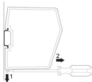
To unmount the module, a screwdriver is needed. Use the screwdriver to push the DIN-rail fastening mechanism on the back of the module down until it locks in a fixed and open position (1). Then unhook the module from the DIN-rail (2).
