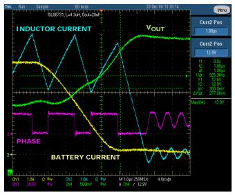
FIGURE 20. OVERVOLTAGE PROTECTION IN ISL88731C
