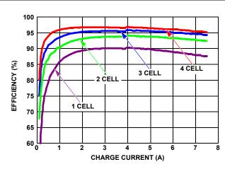
FIGURE 1. EFFICIENCY vs CHARGE CURRENT AND BATTERY VOLTAGE (EFFICIENCY DCIN = 20V)
