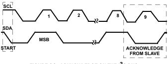
FIGURE 24. ACKNOWLEDGE ON THE I<sup>2</sup>C BUS
