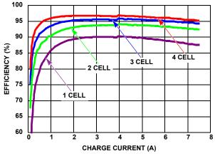
FIGURE 8. EFFICIENCY vs CHARGE CURRENT AND BATTERY **VOLTAGE (EFFICIENCY DCIN = 20V)**
