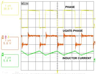
FIGURE 14. SWITCHING WAVEFORMS IN CC MODE
