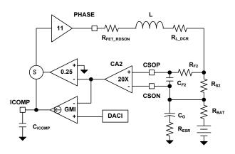
FIGURE 27. CHARGE CURRENT LIMIT LOOP
