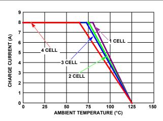
FIGURE 2. DERATING CURVE WITH NATURAL AIR FLOW (MEASURED ON 10cm x 10cm EVALUATION BOARD)
