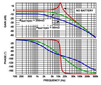
FIGURE 31. FREQUENCY RESPONSE OF THE LC OUTPUT FILTER
