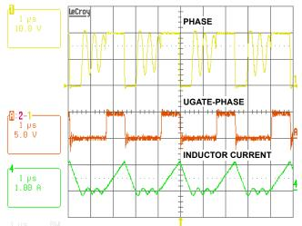
FIGURE 13. SWITCHING WAVEFORMS IN DIODE EMULATION MODE
