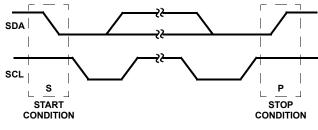
FIGURE 23. START AND STOP WAVEFORMS
