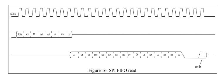
After the last read or write transaction, the SPI master will set the SCL signal back to its idle state (LOW).
