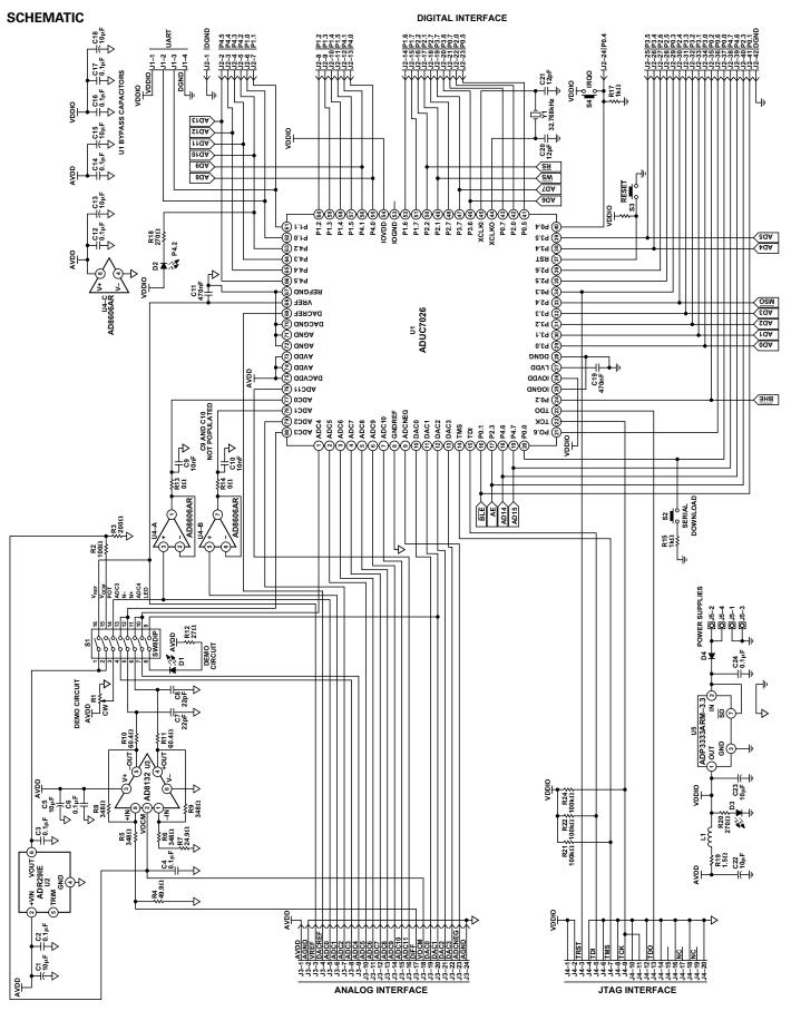
Figure 4. ADuC7026 Evaluation Board Schematic
