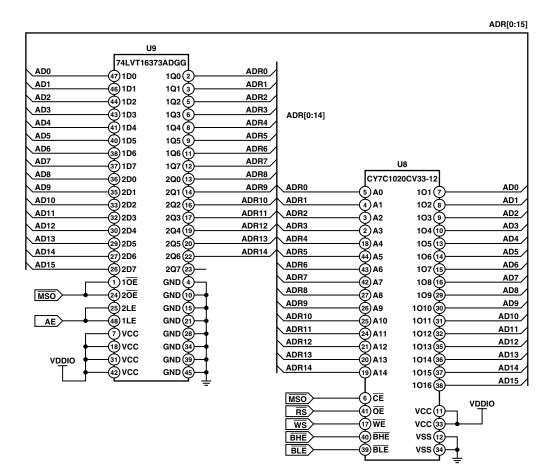
Figure 2. External Memory Connections
