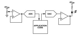
Figure 3. Circuit Diagram of the RTD Circuit
