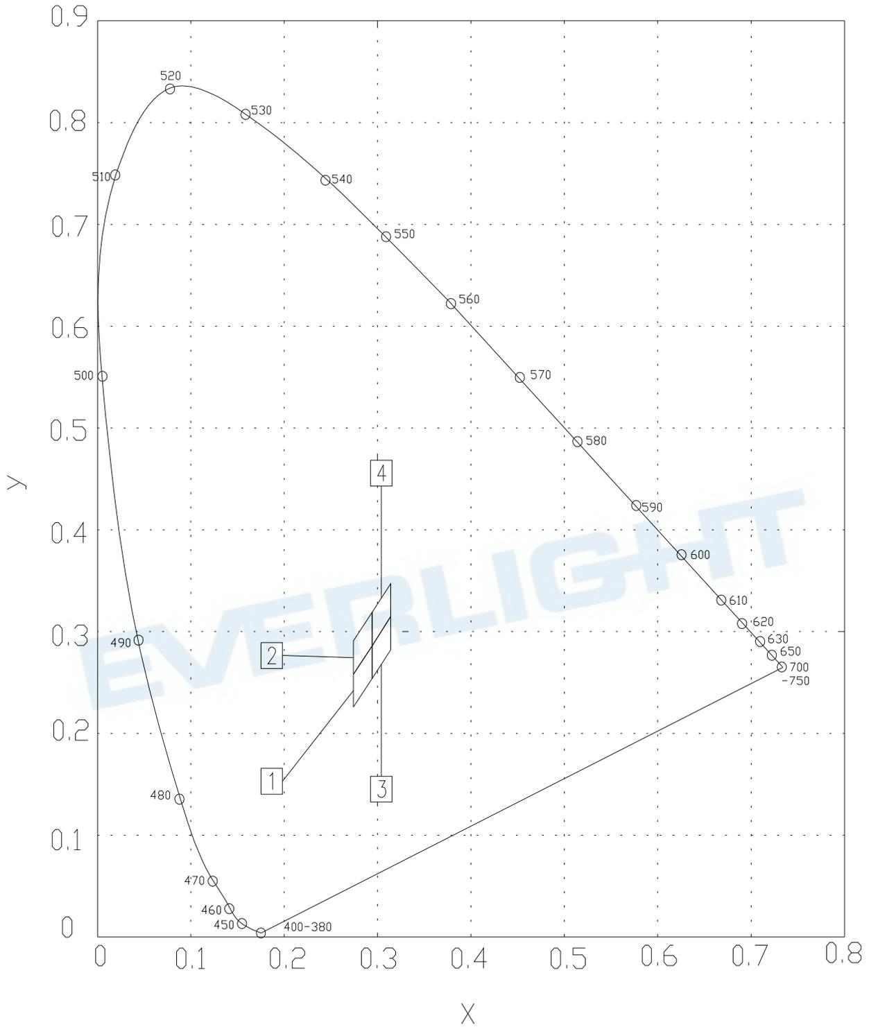
Typical Electro-Optical Characteristics Curves
