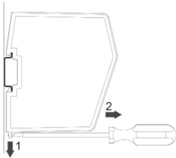
To unmount the module, use a screwdriver to push the DIN-rail fastening mechanism on the back of the module down until it locks in a fixed and open position (1). Then unhook the module from the DIN-rail (2).
