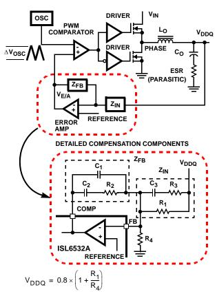
FIGURE 5. VOLTAGE-MODE BUCK CONVERTER
