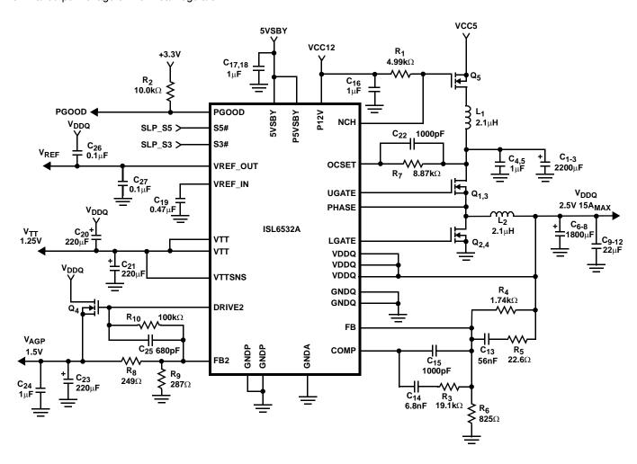
FIGURE 8. DDR SDRAM AND AGP VOLTAGE REGULATOR USING THE ISL6532A
