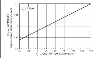
Figure 7. Breakdown Voltage Variation with Temperature.
