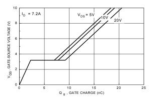
Figure 10. Gate Charge Characteristics.
