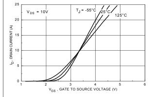
Figure 5. Transfer Characteristics.
