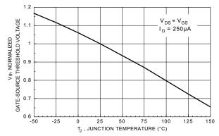
Figure 6. Gate Threshold Variation with Temperature.
