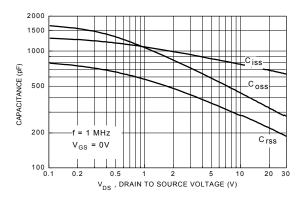
Figure 9. Capacitance Characteristics.
