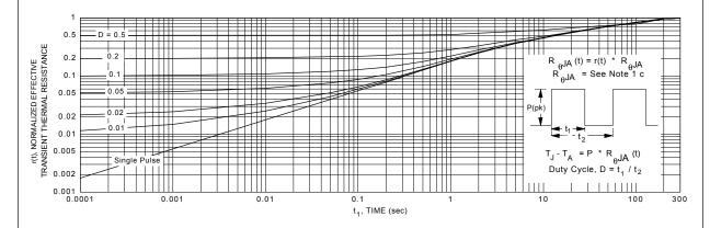
Figure 15. Transient Thermal Response Curve.
