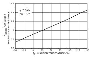
Figure 3. On-Resistance Variation with Temperature.
