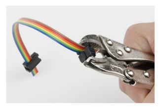
Finally, assemble the additional connectors to the ends of the other ribbon cables, as shown below. Orientation of the connector is important, as the keying on the shrouded headers forces them into the proper orientation only if the cables are assembled right!
