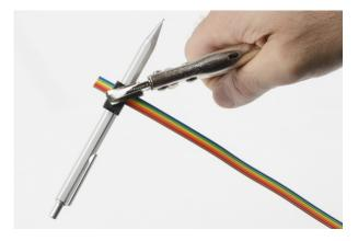
Next, we'll want to crimp on one of the other connectors. See the image below for proper orientation; crimping this in place is much easier because it doesn't have pins to be damaged.
