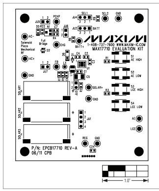
Figure 3. MAX17710 EV Kit Component Placement Guide— Component Side
