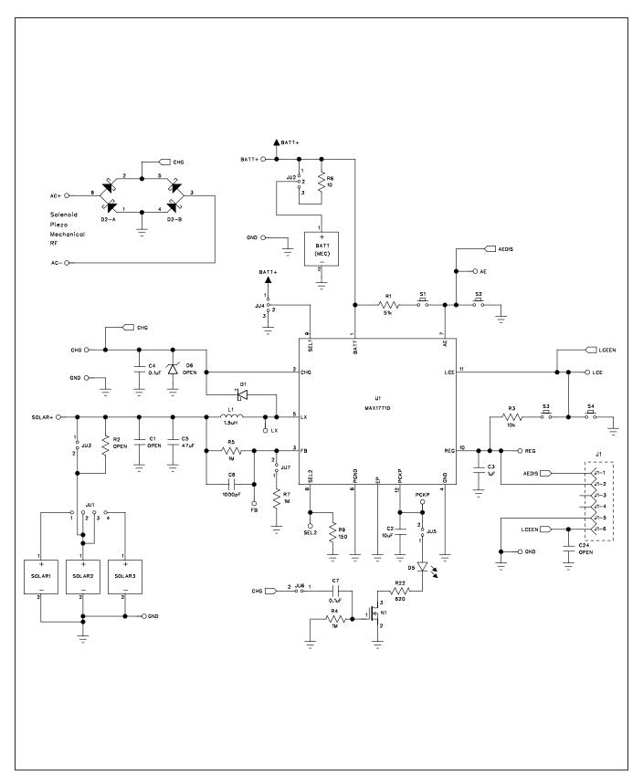
Figure 2. MAX17710 EV Kit Schematic
