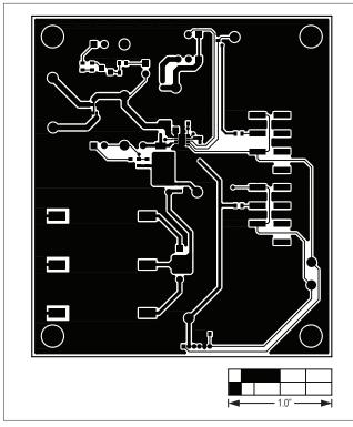
Figure 4. MAX17710 EV Kit PCB Layout—Component Side
