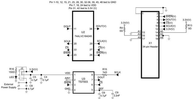
Figure 5. TS7003 Evaluation Board Circuit
