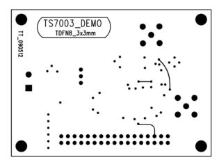
Figure 8. Bottom Layer (GND)
