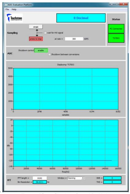
Figure 4. TS7003 Shutdown Control Enabled
