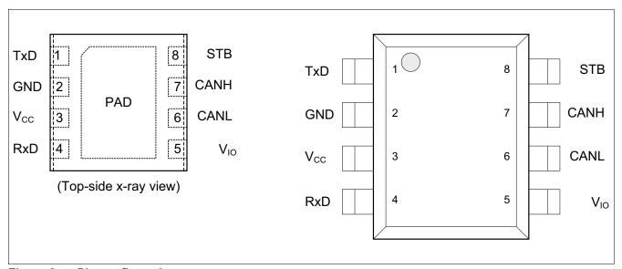
Figure 2 Pin configuration
