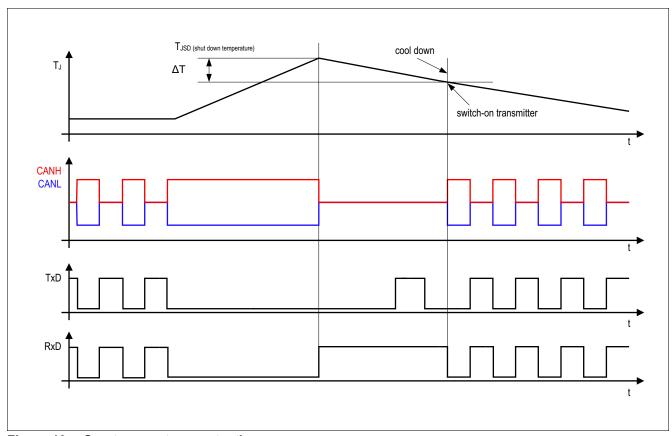
Figure 10 Overtemperature protection
