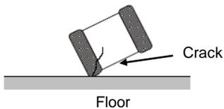
3. When printed circuit boards are piled up or handled, the corner of another printed circuit board should not be allowed to hit the capacitor in order to avoid a crack or other damage to the capacitor.
