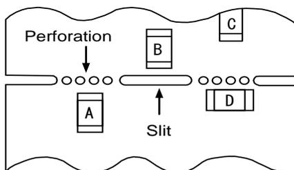
[Mounting Capacitors Near Screw Holes]
