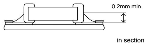
**Inverting the PCB** Make sure not to impose any abnormal mechanical shocks to the PCB.
