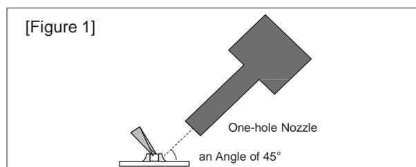
3. Optimum solder amount when re-working with a soldering iron
