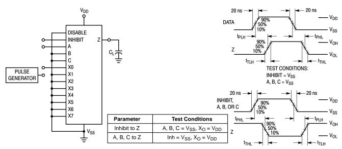
Figure 2. AC Test Circuit and Waveforms
