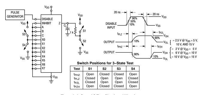
Figure 3. 3-State AC Test Circuit and Waveform
