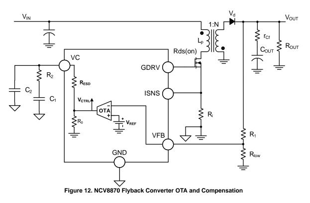
The following equations may be used to select compensation components  $R_2$ ,  $C_1$ ,  $C_2$  for Figures 11 & 12 power supply. Required input design parameters for analysis are:
