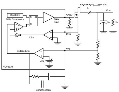
Figure 10. Current Mode Control Schematic
