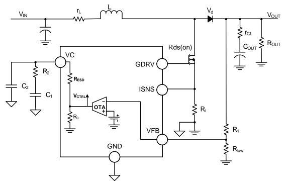
Figure 11. NCV8870 Boost Converter OTA and Compensation
