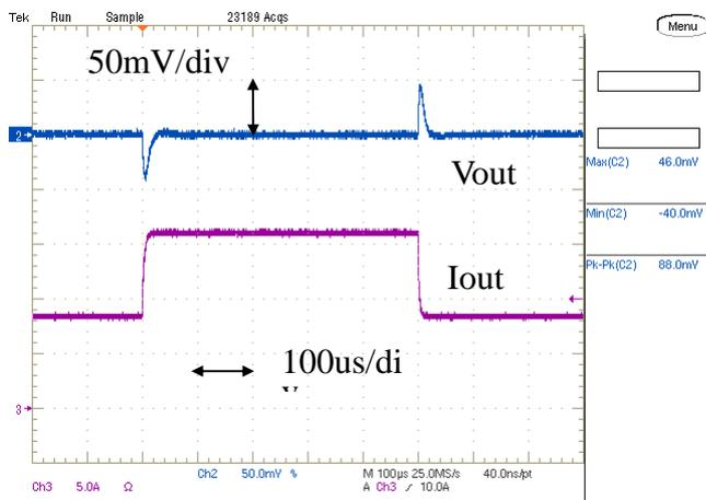
Fig.12-1a. Load Transient Response ( $V_{out}:1.8V$ )
