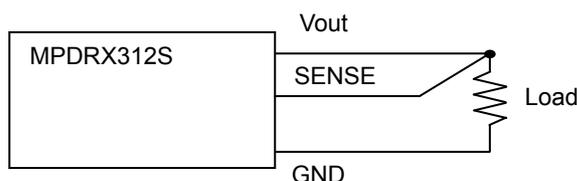
Please do NOT connect SENSE-pin to the output of LC filter that is set to the Vout line. When using this way, this product will not operate properly.
