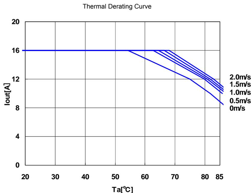
The above derating limits apply to this product soldered directly to 101.6\*180mm\*1.6mm PCB. Any adjacent parts of high temperature may cause overheating. For reliable operation, please ensure that the FET temperature of this product is maintained below 120°C and the inductor temperature is below 106°C.
