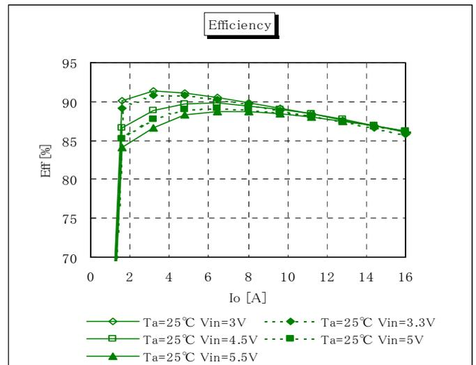
Fig.12-3-2. Efficiency v.s. Output Current
