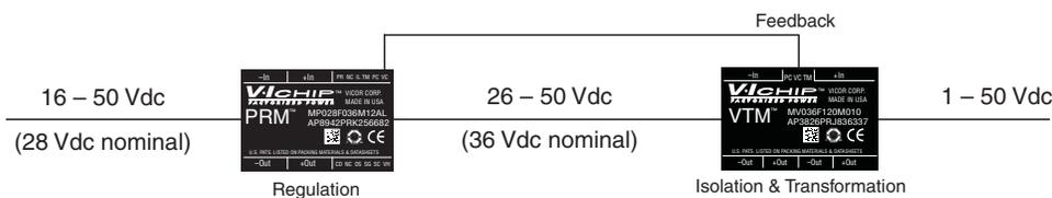
Together, the PRM and the VTM chip set provides the full functionality of a DC-DC converter, but with breakthrough performance and flexibility in a rugged, miniature package.
