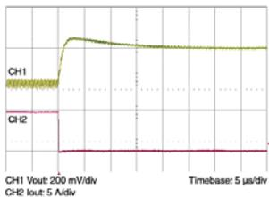
Load step with 100 μF input capacitance and no output capacitance (MV036F120M010)
