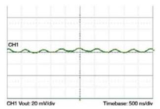
28 V to 12 V, 10 A VTM with 4.7 μF external capacitance
