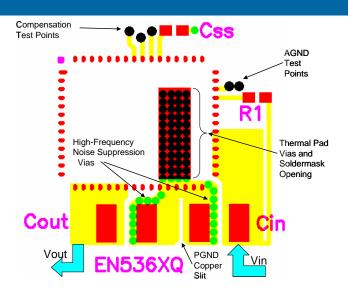
Figure 6. Use of thermal & noise suppression vias.
