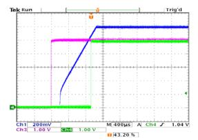
Start up waveforms  $V_{IN}$ =5.0V,  $V_{OUT}$ =1.2V,  $C_{SS}$ =15nF, Ch 1 =  $V_{OUT}$ , Ch 3 = ENABLE, Ch 4 = POK.
