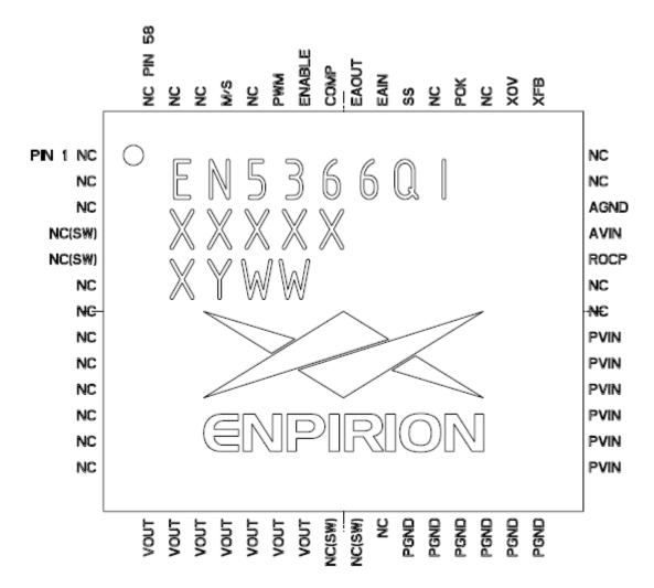
Figure 2. Pin Diagram, top view.
