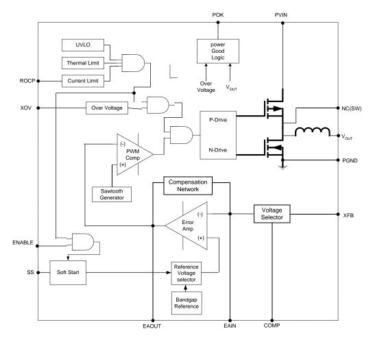
Figure 3. System block diagram.
