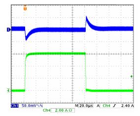
Transient Response  $5.5V_{\text{IN}}/1.2V_{\text{OUT}},\,0\text{-}6A,\,10\text{A}/\text{uS}.$   $C_{\text{OUT}}\text{=}50\text{uF}.$
