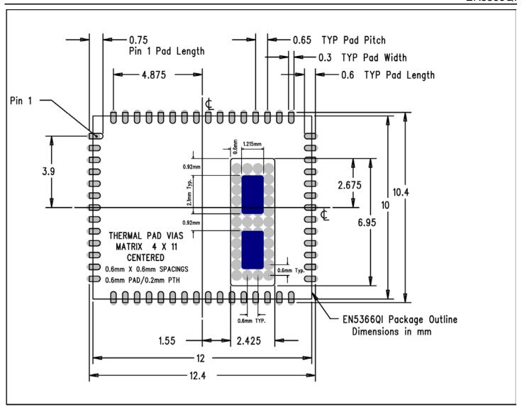
Figure 8: EN5366QI PCB Footprint (Top View)
