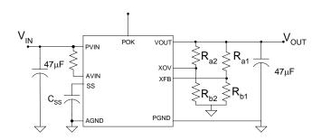
**Figure 4.** V<sub>OUT</sub> and OVP resistor divider networks.
