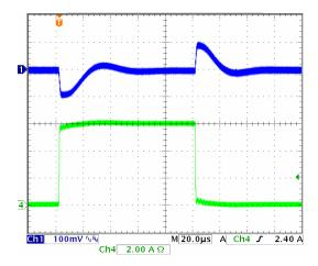
Transient Response  $5.5V_{\text{IN}}/3.3V_{\text{OUT}},~0\text{-}6A,~10A/\text{uS}.$   $C_{\text{OUT}}\text{=}50\text{uF}$
