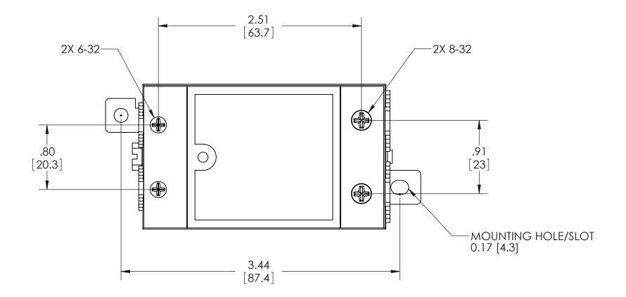
Tolerances: ± 0.02 in / 0.5 mm. All dimensions are in: inches [millimeters]
